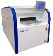
The VAC 745/765 (available as batch or inline) combines the advantages of the vapor phase with the vacuum process and guarantees void-free solder joints with highest quality. The soldering system operates in a completely inert atmosphere during the whole reflow and vacuum process. Many patented features are available and provide a wide range of flexibility. The machine promises oxygen-free soldering an no overheating of components. In addition, the power consumption of the machine is very low.
