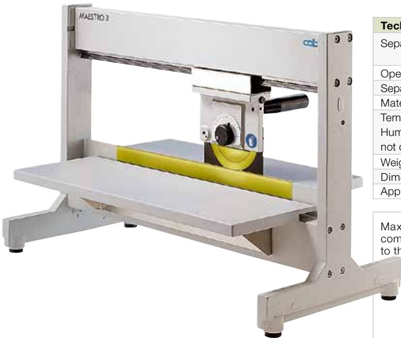
MAESTRO 3E separates both small and large pre-scored PCBs. The table and the rest can be continuously adjusted to the most suitable working position. The slit between the linear blade and the rest can be adjusted to ensure that the side strips fall through and are sorted out.
